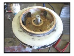
The impeller was then MACHINED back to the correct size and profile.
