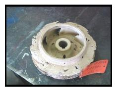
This impeller arrived in our Dutch Distributors workshop from a MAJOR shipping company. It was on-board a tanker and required IMMEDIATE attention. You can see from the EXCESSIVE damage that a MAJOR repair would have to be undertaken OR the impeller replaced. The impeller was made from BRONZE and damage had been caused by SERIOUS cavitation.
